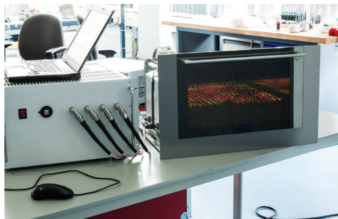
Ampleon demo system showing an LED tri-colour field detector board in use
